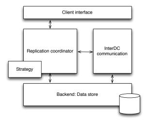
Figure 4: Architecture of the Adaptive Replication component.
